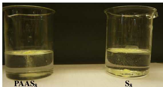
Figure 7.2 Wetting behaviors of PAAS 8 and uncoated sulfur in ethylene glycol.
